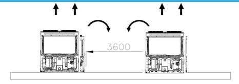
For mutliple chiller installation it is recommended to install the chillers is a single row as hown in the picture below
