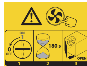
Danger of running fans
